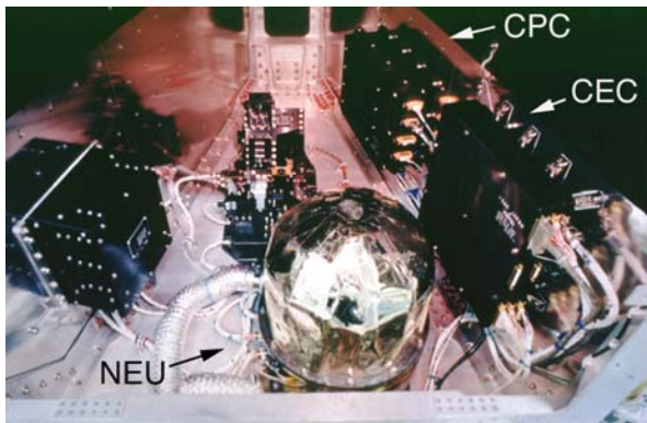
Fig. 2 BIO experiment system installed on Special Payload Unit-2. NEU: Pressurized container of Newt Experiment Unit, CEC: Experiment dedicated computer to interface data and command, and CPC: Power controller.
